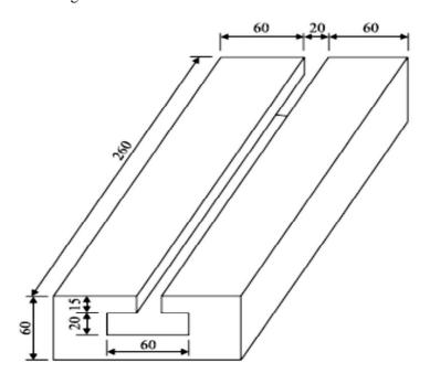
**Step II**: Cut T-slot of dimensions  $60 \times 20$  with a T-slot cutter Here dia of cutter = 60 mm
