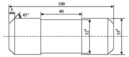
Solution: Ist operation: Turning from £ 38 mm to £ 35 mm
