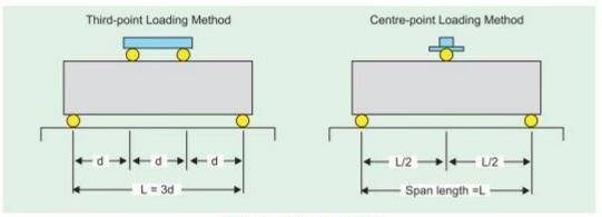
Principles of flexural testing
