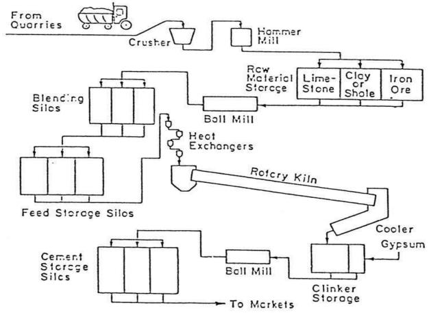
The raw materials used for manufacturing Portland cement are limestone, clay and Iron ore. a) Limestone (CaCO3) is mainly providing calcium in the form of calcium oxide (CaO)
