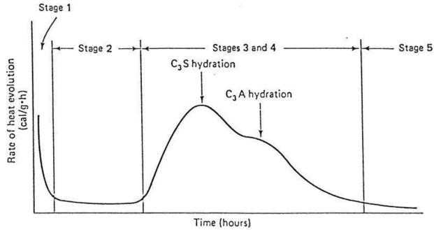
From the figure, five stages can be easily identified. Since C3S is a dominating component in cement, the five stages above can be explained using the reaction process of C3S by the following table.
