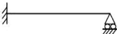
$$i = r - e \text{ where, } r = \text{no of reactions, } e = \text{no of equilibrium conditions} \\ r = 4 \text{ and } e = 3 \\ i = 4 - 3 = 1$$
