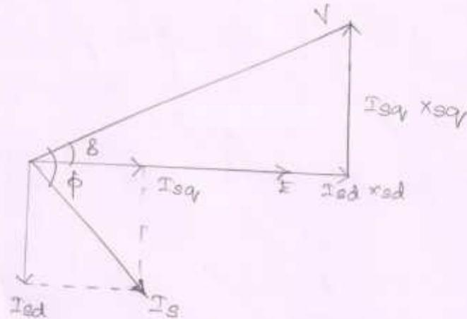
4. Derive the torque equation of synchronous reluctance motor.
