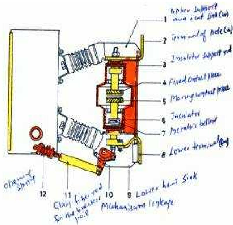
Cross sectional view of a typical Vacuum Circuit-breaker (Side View)
