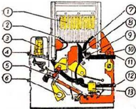
1. Arc chutes having deionization plates coated with plastic paint on the top half.
