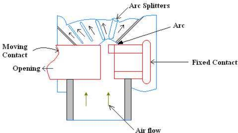
thermal action. The arc ends travel along the Arc Runner (Arcing horns). The arc moves upwards and is split by arc splitter plates (5). The arc is extinguished by lengthening, cooling, splitting etc. In some breakers the arc is
