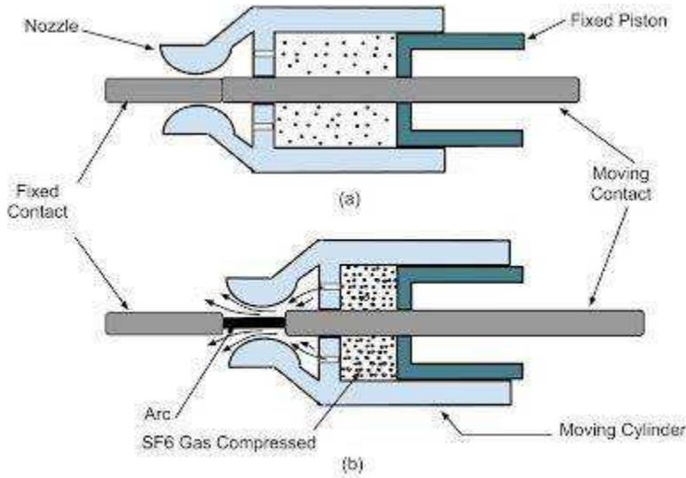
Fig-A: Puffer Type SF<sub>6</sub> Circuit Breaker
