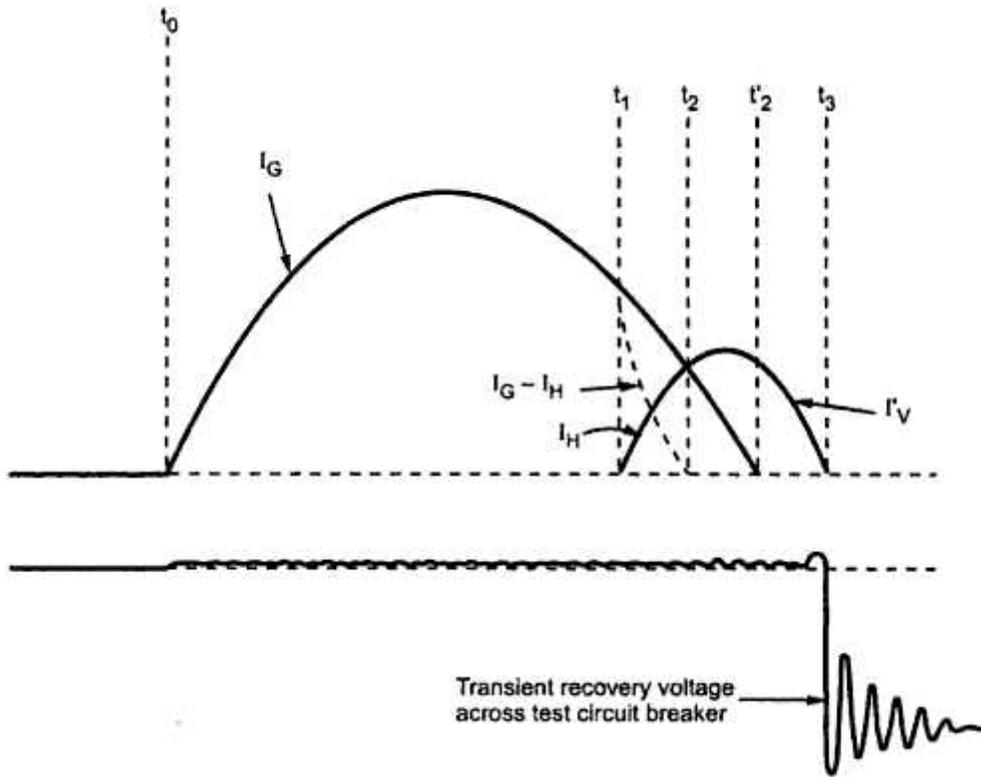
**Series injection method waveforms**
