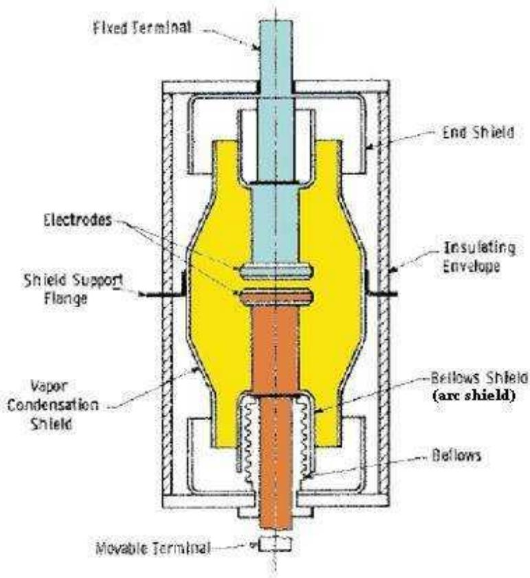
Representation of vacuum interrupter chamber in vacuum circuit breaker
