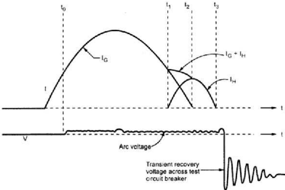
(b) Parallel current injection method waveforms
