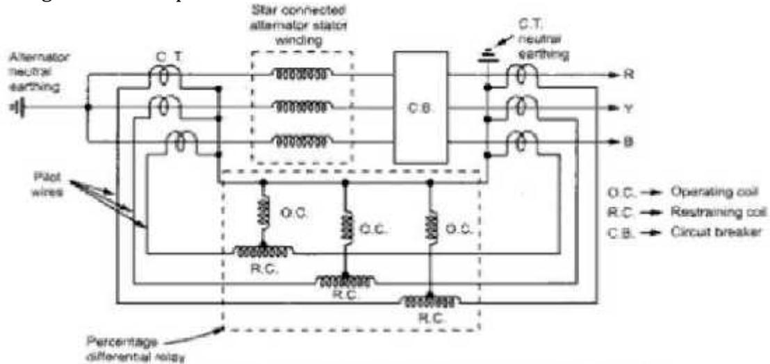
**Fig. Merz-Price protection for star connected alternator**
