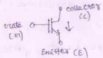
→ structure of IGBT → Diagram & Explanation
