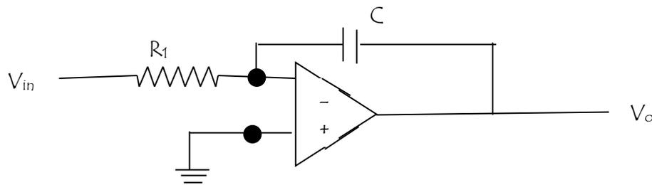
A basic integrator is shown above.  $V_o(t) = -1/R_1C \int V_{in}(t) dt + V_o(0)$
