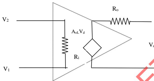
It can be seen that op-amp is a voltage controlled voltage source and  $A_{OL} V_d$  is an equivalent Thevenin voltage source and  $R_o$  is the Thevenin equivalent resistance looking back into the output terminal of an op-amp.
