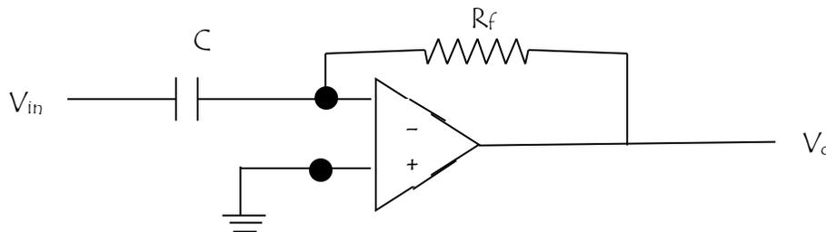
A basic differentiator is shown above.  $V_o = -R_fC dV_{in}/dt$
