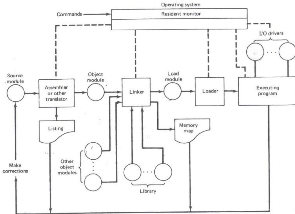
The DOS linking program links the different object modules of a source program and function library routines to generate an integrated executable code of the source program. The main input to the linker is the .OBJ file that contains the object modules of the source programs. Other supporting information may be obtained from the files generated by the MASM. The linker program is invoked using the following options.
