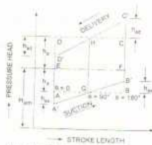
Fig. 20.5 Effect of acceleration on indicator diagram.
