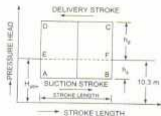
Fig. 20.4 Ideal indicator diagram.
