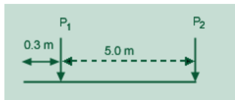
Fig. 4.51 Loading on combined footing
