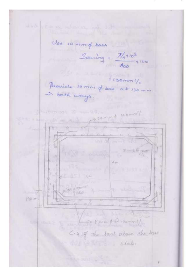
Design a runfaced (re) water tank of in dimerción 10 x 3 mx 3. The tant is to be pe under ground. The Soil Savaunding earth likely to get wet. The angle senone is 30° at dry condition and 6° at wet. Take density of Sail as 20 KN/m2, adopt mso grade I midd that box's. given: Sire = 10 m x 3 m x 3 m. Angle of super @ day state = 30° Unit wil of Sail = 20 KA/m2 H20 + grade I ms boxs. is Step 2 permente 1 design coast. Tension du te bending Page No 7 Oct = 17 N/mm2.
