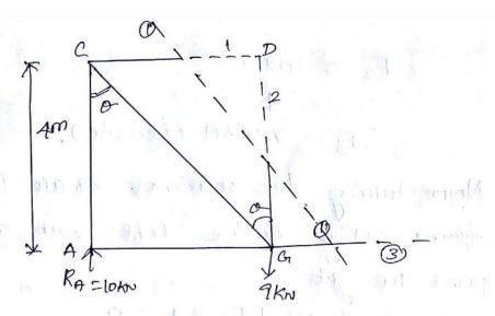
Now draw a section line 0-0 cutting the to be determined consider the quilibrium of the left part of the truss (because it is smaller then the right Part). The part is shown in figure. Let F, F2 and F3 are the forces members about 1, 2 and 3 respectively. Let their directions are assumed as shown in figure. Taking moments of all the forces actings on the lebt part about point o,
