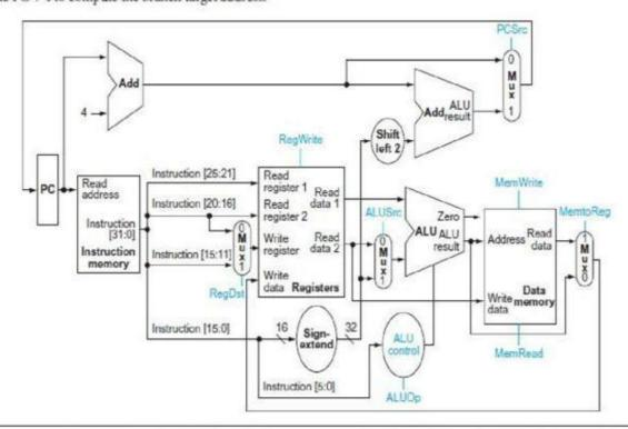
The datapath of Figure 4.11 with all necessary multiplexors and all control lines identified. The control lines are shown in color. The ALU control block has also been added. The PC does not require a write control, since it is written once at the end of every clock cycle: the branch control logic determines whether it is written with the incremented PC or the branch target address.
