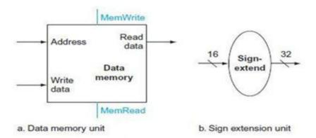
The two units needed to implement loads and stores, in addition to the register file and ALU of , are the data memory unit and the sign extension unit.
