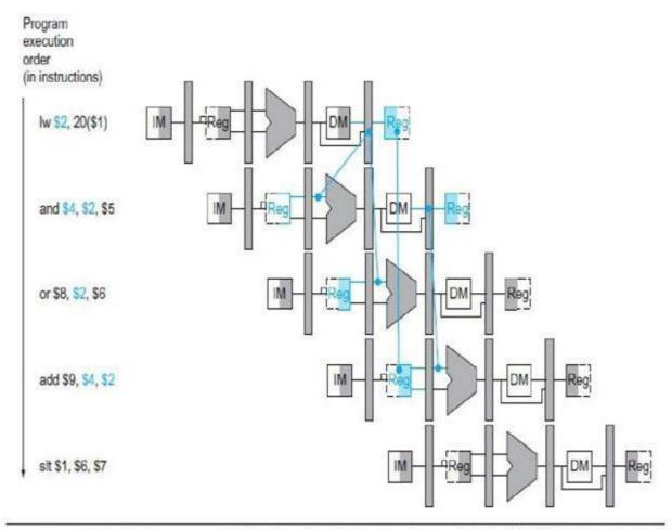
A pipelined sequence of instructions. Since the dependence between the load and the following instruction (and) goes backward in time, this hazard cannot be solved by forwarding. Hence, this combination must result in a stall by the hazard detection unit.
