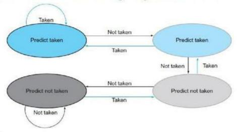
The states in a 2-bit prediction scheme. By using 2 bits rather than 1, a branch that strongly favors taken or not taken—as many branches do—will be mispredicted only once. The 2 bits are used to encode the four states in the system. The 2-bit scheme is a general instance of a counter-based predictor, which is incremented when the prediction is accurate and decremented otherwise, and uses the mid-point of its range as the division between taken and not taken.
