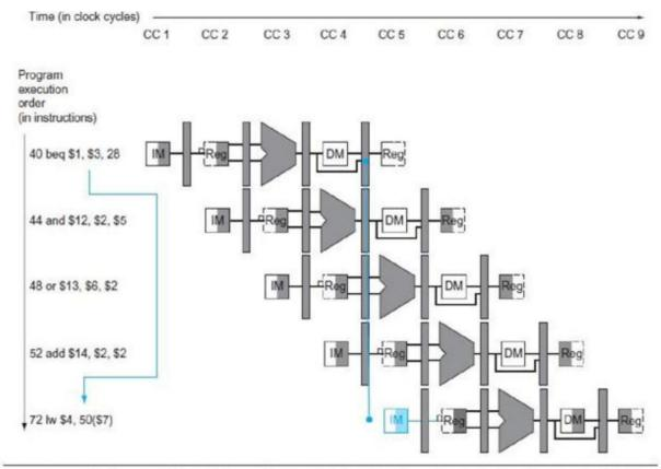
The impact of the pipeline on the branch instruction. The numbers to the left of the instruction (40, 44, ...) are the addresses of the instructions. Since the branch instruction decides whether to branch in the MEM stage—clock cycle 4 for the beq instruction above—the three sequential instructions that follow the branch will be fetched and begin execution. Without intervention, those three following instructions will begin execution before beq branches to
