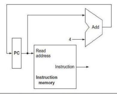
A portion of the datapath used for fetching instructions and incrementing the program counter. The fetched instruction is used by other parts of the datapath.
