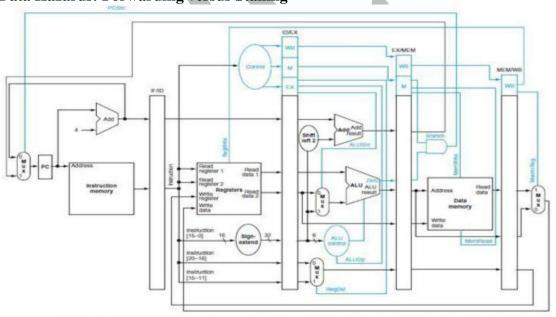
. The pipelined datapath of , with the control signals connected to the control portions of the pipeline registers. The control values for the last three stages are created during the instruction decode stage and then placed in the ID/EX pipeline register. The control lines for each pipe stage are used, and remaining control lines are then passed to the next pipeline stage.
